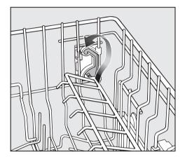
Pull the cup rack upwards and click it back into position at the required height.
